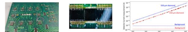
150 channels 9x1 sCVD mosaic \mu\text{strips} diamonds + integrated FE electronics (QDC) CMOS 130 nm
