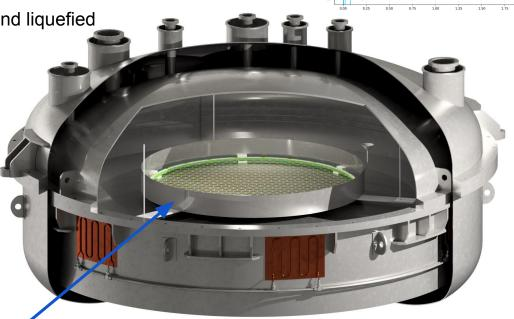
bathtub  $\varnothing$  = 1.5m  $\rightarrow$  reach higher liquid level,necessary to submerge test components in LXe
