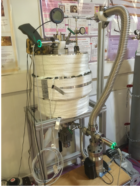
SPC-1 (2018) D = 0.4 m r_{\text{ball}} = 1 \text{ mm} (1 bar)
