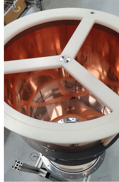
CPC-20 (2022) L x D = 1 x 0.37 (m) r_{\text{wire}} = 20 \mu\text{m} (1 bar)
