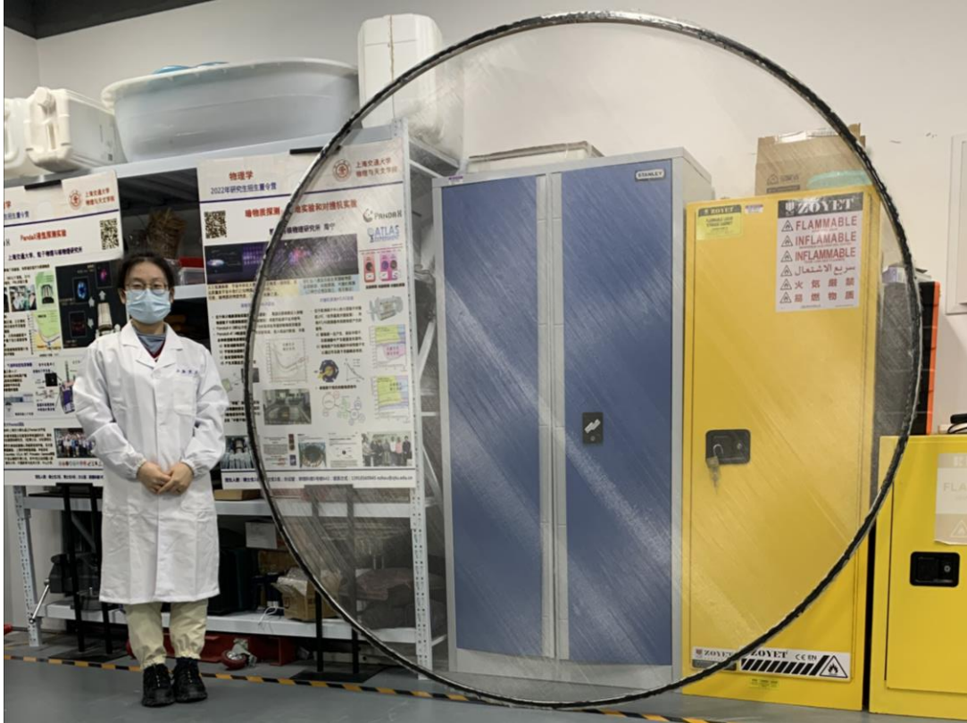
TPC: Large size high light transmission electrode
