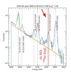
LZ obtained an unprecedented energy resolution for liquid xenon at high energies:
