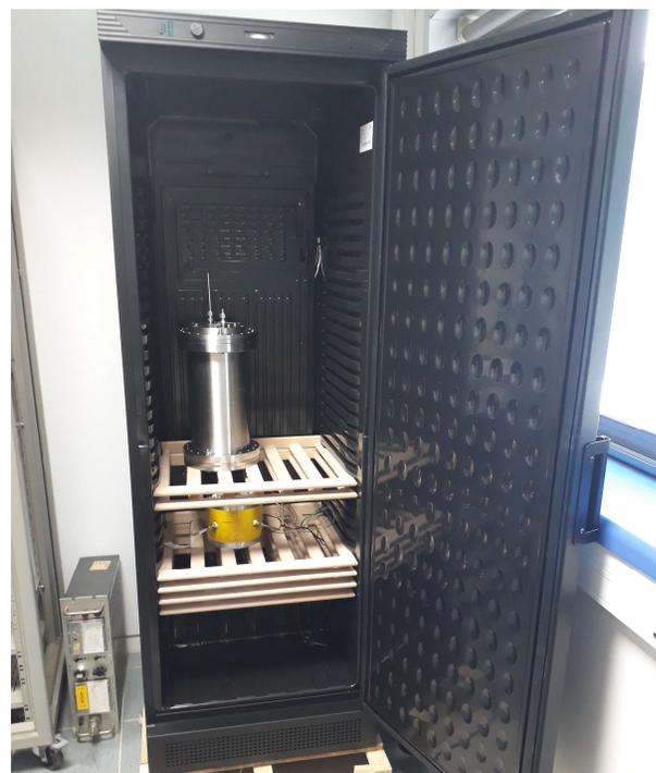
Radon chamber in climatic chamber .
