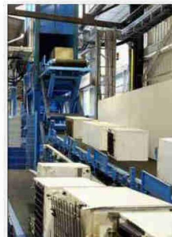
« Phase 2 » : shredding under inert atmosphere, suction of the gas in the insulation foams
