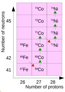
β<sup>-</sup> disintegrations Neutron capture
