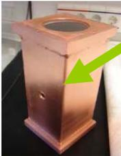
Mylar window at ANAIS-0 allows low energy calibrations
