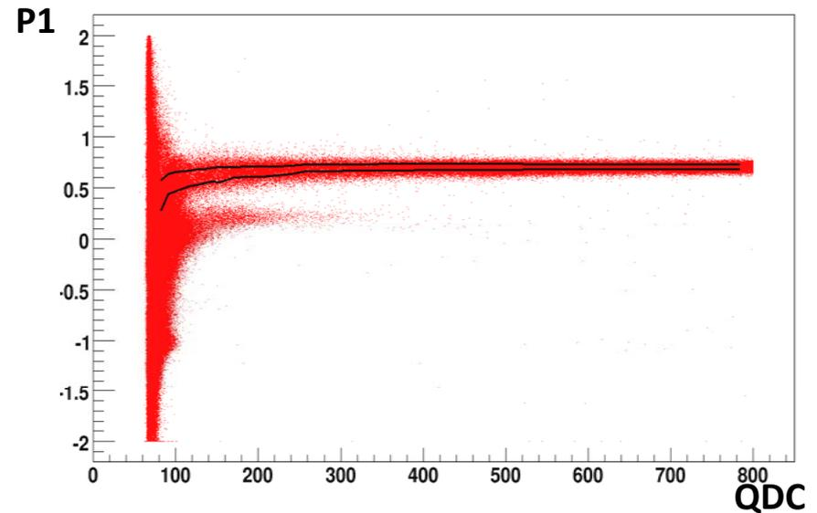
Average of the P1 values for the two PMT signals of ANAIS-0 when exposing the detector to a  $^{57}\text{Co}$  source: population of bulk scintillation events (left) and background events (right). Solid line shows the  $1\sigma$  region about the mean value of the parameter for calibration events.
