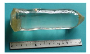
We are going to measure radioactive contamination of the 3<sup>rd</sup> sample in scintillation mode to estimate how concentration of Th, U, Ra, K depends on crystal growth
