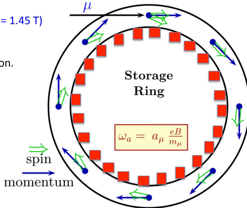
1. Measure  $e^+$  with  $E > 1.9 \text{ GeV}$  in 24 calorimeters vs time (30  $\mu\text{s}$  after injection)
