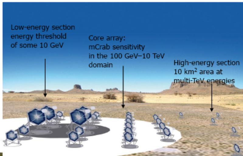
An array of > 60 telescopes of 3 classes for a wide energy range of sensitivity
