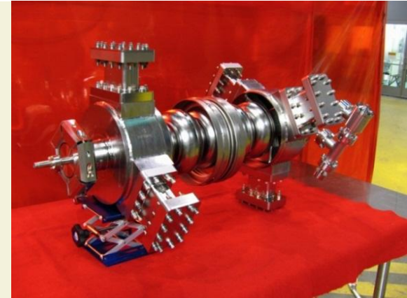
High current cavity for ERL/FEL (JLab) 1.5GHz
