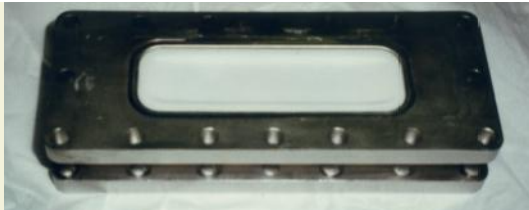
1.5GHz, 2.5kW rectangular WG RF window (TiO 2 ceramics)
