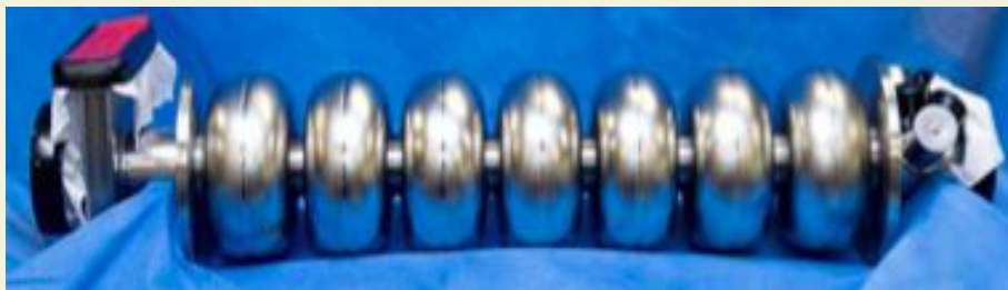
CEBAF upgrade 7-cell cavity (JLab) 1.5GHz
