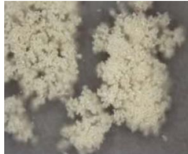
Sulphur removed from a PVDF tube
