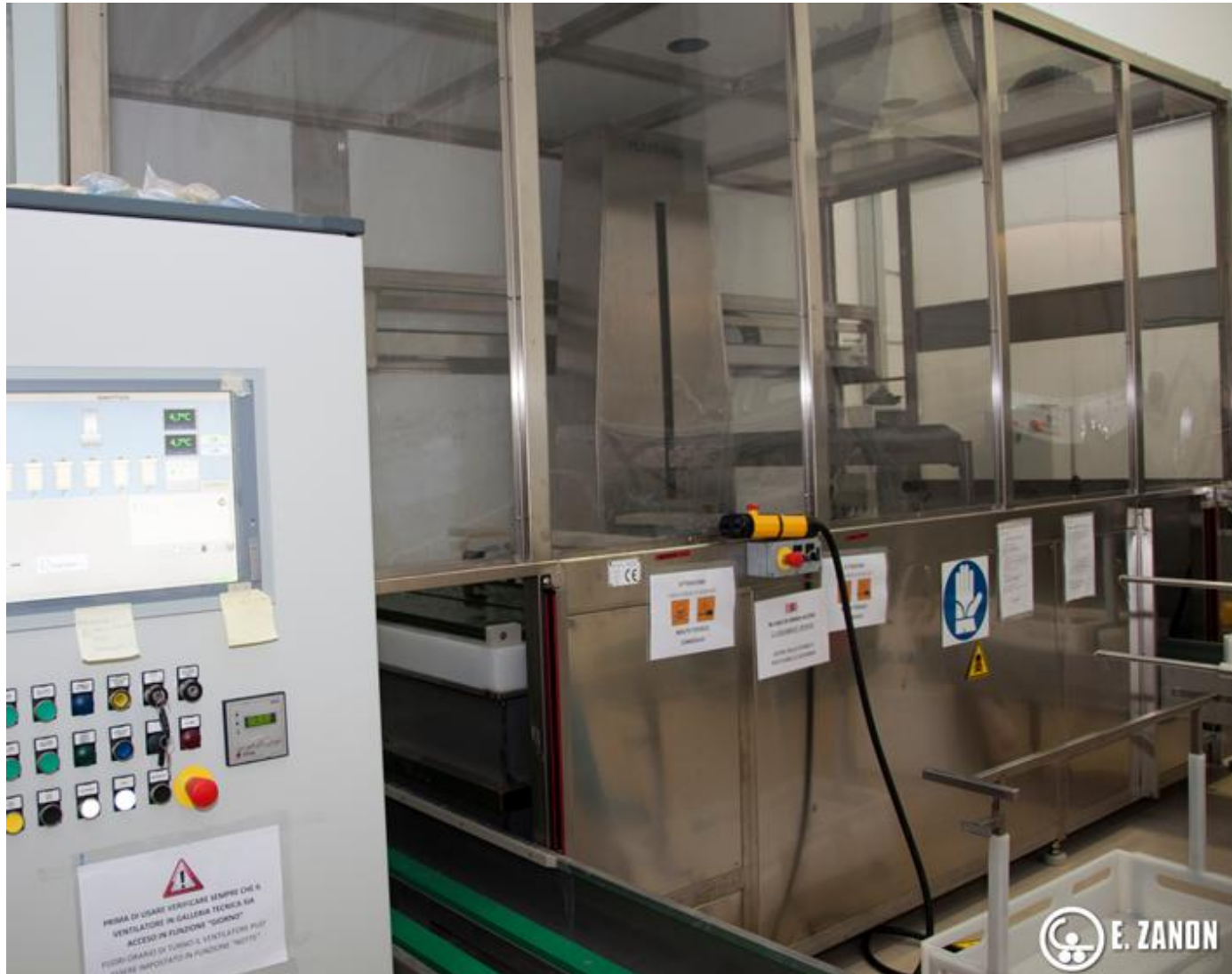
Automatic BCP system for subcomponents @ Ettore Zanon for EXFEL (etching + rinsing)
