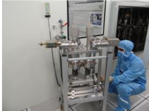
Leak test after reception
