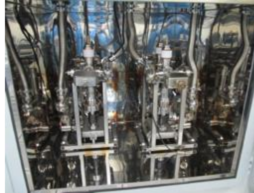
75h baking cycle at 130°C
