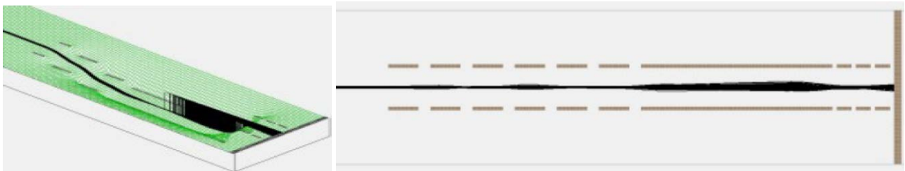
Trajectory simulations showing (right) the single-stage version shown as a potential surface (the effect of pulsing the voltage on the drift tube can be seen) and (left) in 2D showing a new, two-stage deceleration geometry (two sets of three electrodes) followed by the pulsed drift tube cavity (long tube), followed by a modular Einzel lens for focusing the antiproton beam into the antihydrogen formation chamber.
