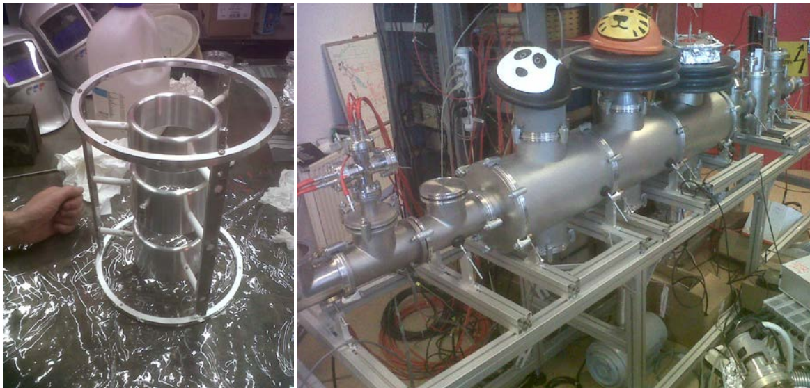
Photographs of the proton-decelerator test bench: (left) one of the two sets of deceleration electrodes; (right) part of the beamline showing the three chambers that house the electrodes; feedthroughs are mounted on insulators for the final deceleration electrode and pulsed drift tube (under the high-voltage protective covers).
