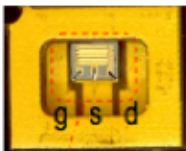
Figure 2 – HEMT in its SOT23 holder.
