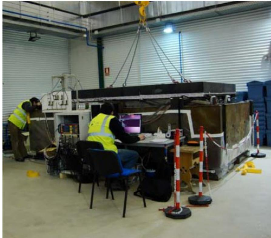
Full BiPo-3 detector inside the shield with separate acquisition for each module
