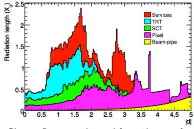
Material distribution at the exit of the inner detector of ATLAS as a function of  $|\eta|$
