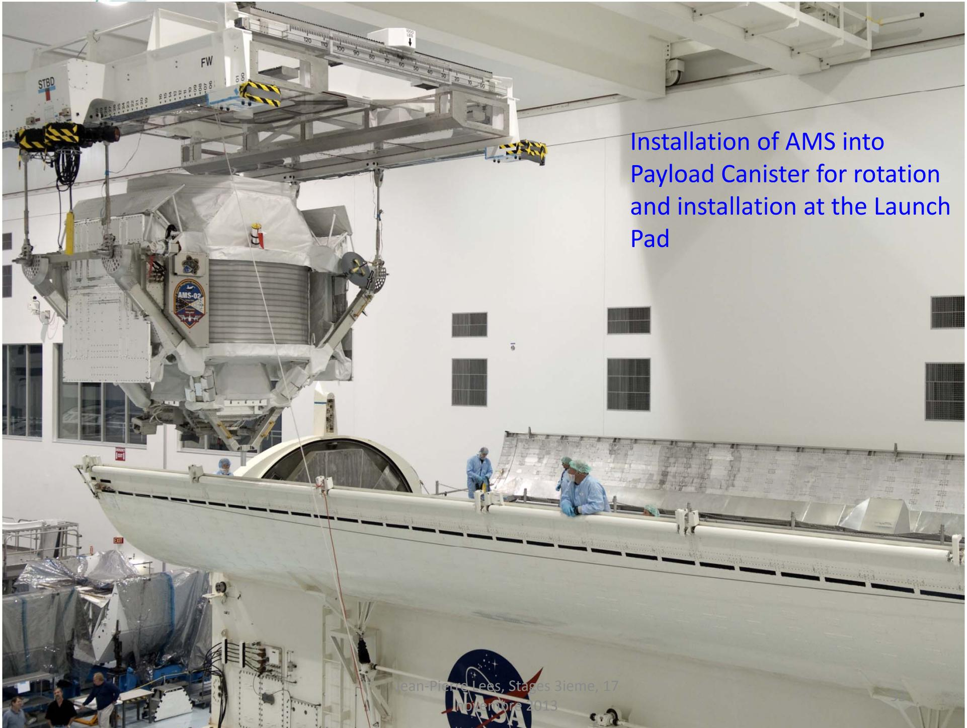
Installation of AMS into Payload Canister for rotation and installation at the Launch Pad
