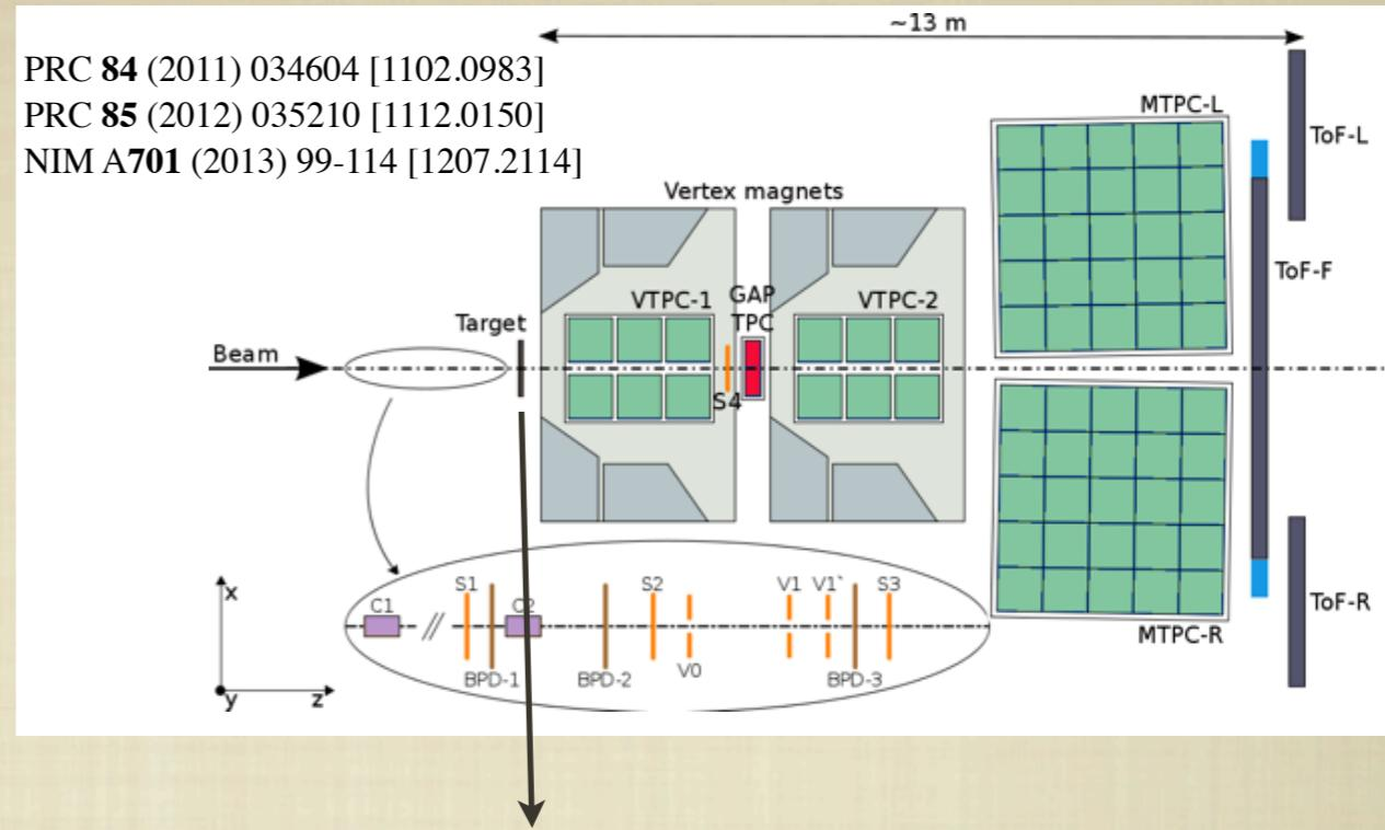
2 targets: thin target and T2K target
