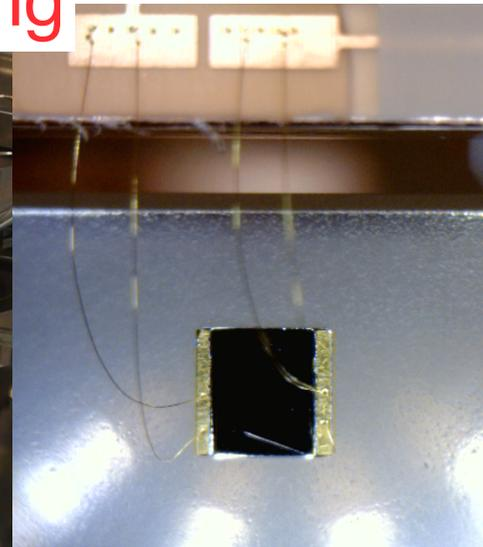
All steps of the assembly performed under nitrogen atmospheres inside glove boxes<sub>8</sub>
