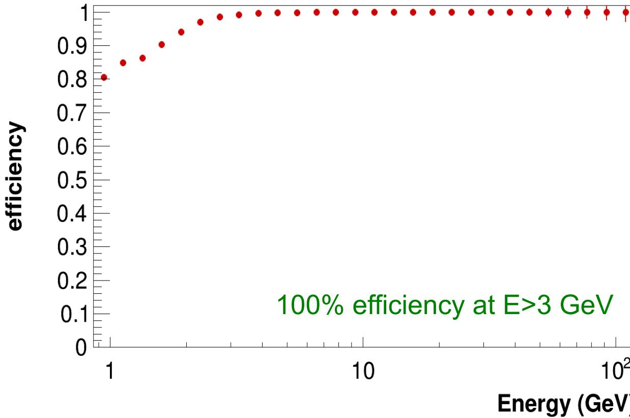
The trigger efficiency has been determined with ISS data using the “unbiased trigger” (a trigger with looser conditions, pre-scaled by 1/100)
