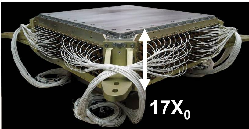
A precision, 3-D measurement of the directions and energies of gammas and electrons up to 1 TeV
