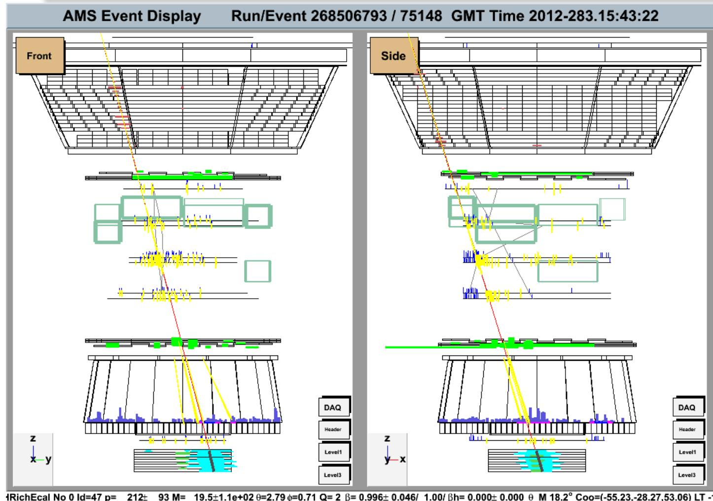
38 GeV electron reconstructed as 0.8 GeV positron.
