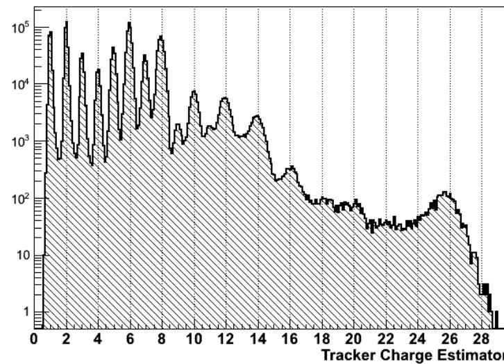
The first layer (L1), used as a standalone charge detector has a charge resolution ( $\sim 0.3$  c.u.) that allows the identification of the fragmentations, being at the top of the instrument (TOI)
