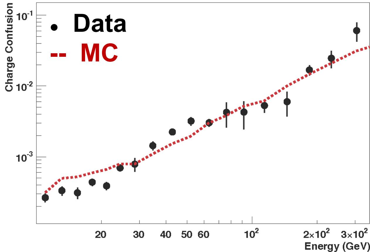
Two sources: large angle scattering and production of secondary tracks along the path of the primary track. Both are well reproduced by MC. Systematic errors correspond to variations of these effects within their statistical limits.
