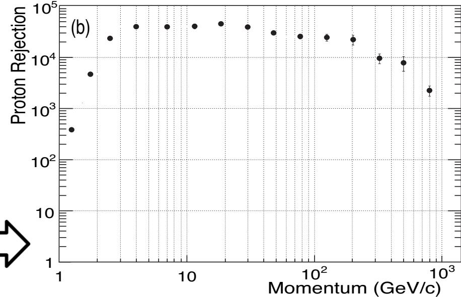
The Calorimeter thanks to its shower shape imaging capabilities can discriminate very sensibly electromagnetic from hadronic showers
