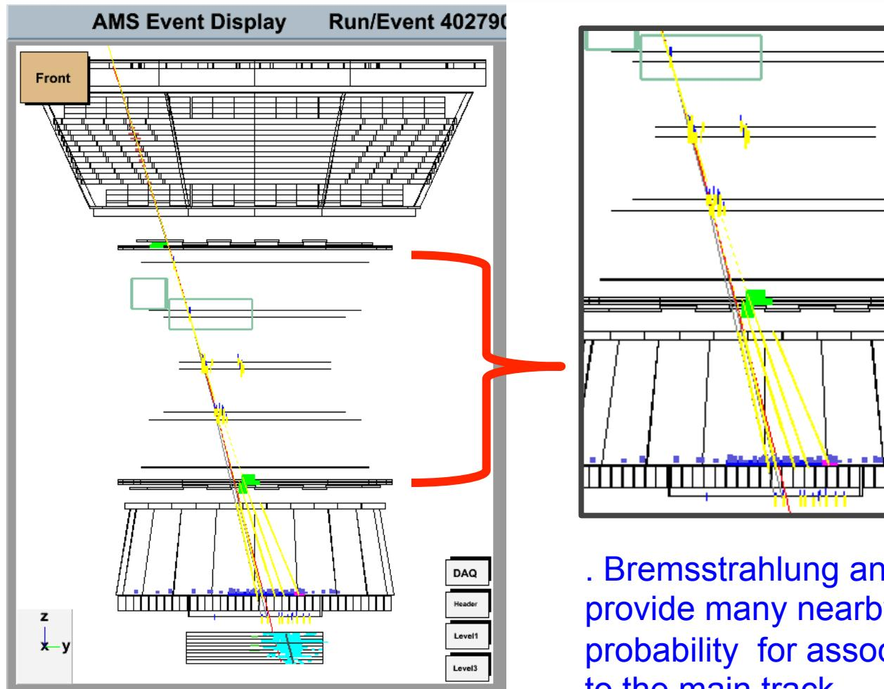
. Bremsstrahlung and delta rays provide many nearby tracks with high probability for association of a wrong hit to the main track.
