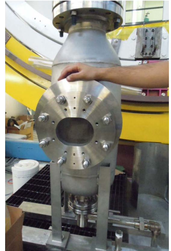
Simplified pressure vessel – \frac{1}{4} the mass of steel as COUPP-4.
