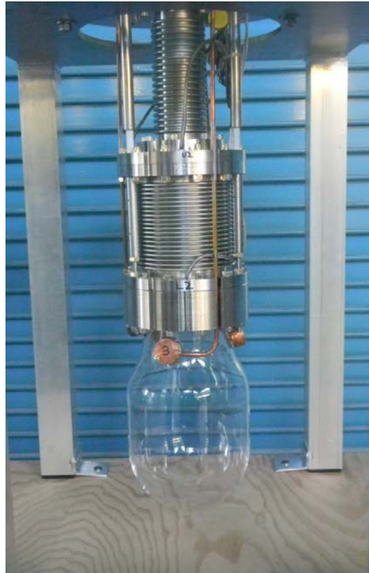
New two-bellows design inner vessel assembly. Silica jar is an exact replica of COUPP-4 jar.
