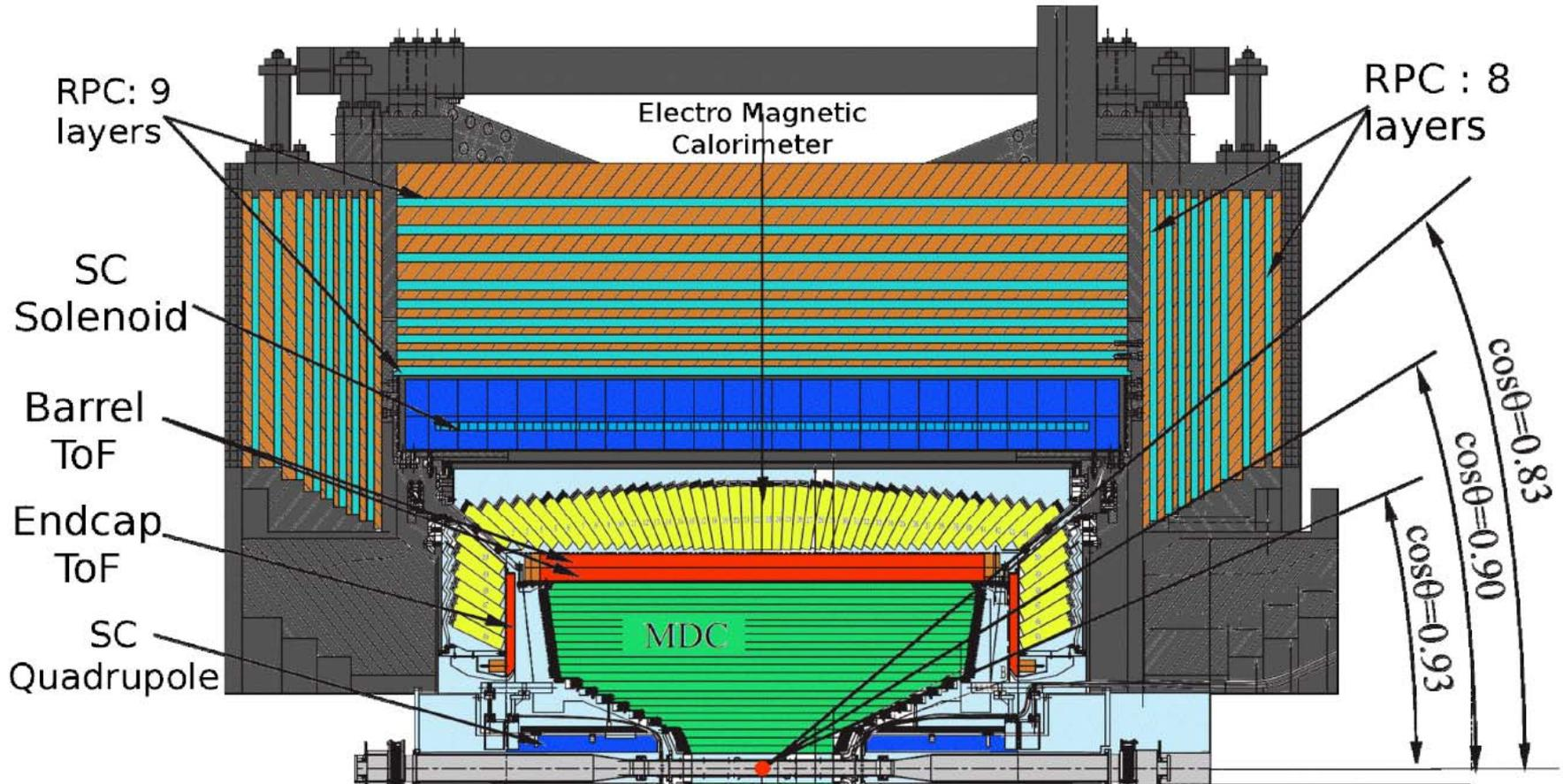
Wire tracker (no Si); TOF +  $dE/dx$  for PID; **CsI Ecal**; RPC muon
