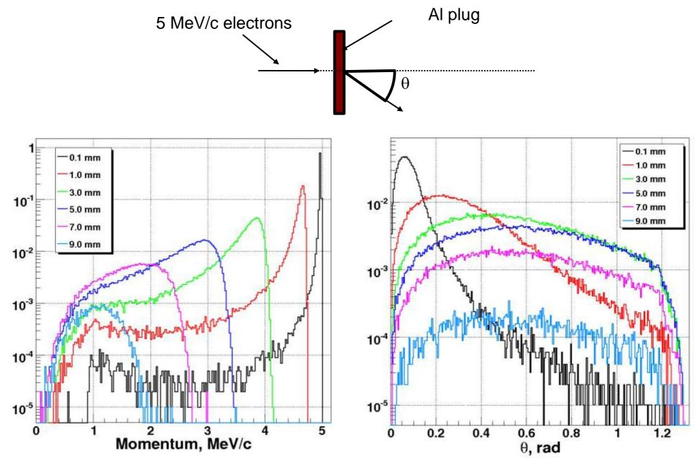
Example of sampling 1 MeV electrons from 5 MeV beam: from simulated 10<sup>8</sup> electrons a sample of ~10<sup>3</sup> electrons and momentum spread of ~10 % are obtained with collimator opening of 6 mm.
