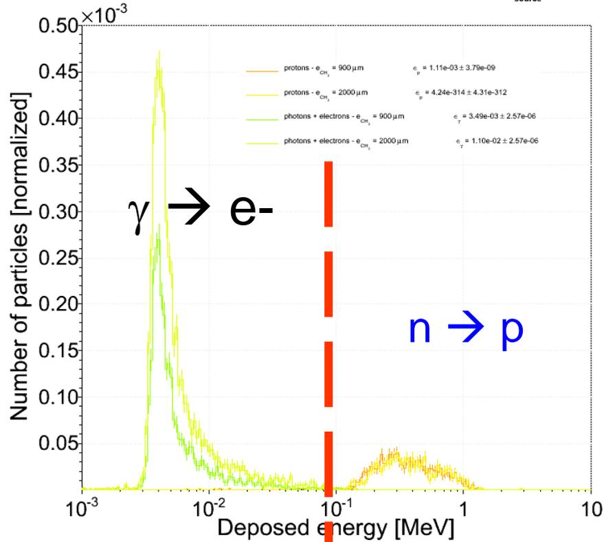
Deposited energy in CMOS sensor calculated by MCNPX 2.6f simulation [nps = 1e6, d<sub>source</sub> = 15 cm]
