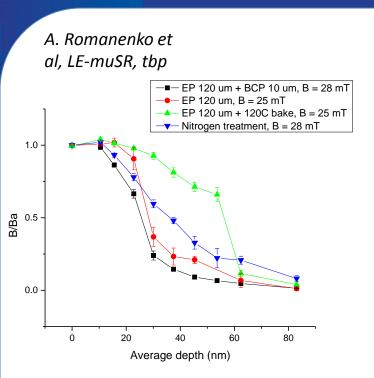
Dead layer due to nanoroughness? Room for Rs improvement if surfaces are mirror smooth (ie <50 nm roughness)?
