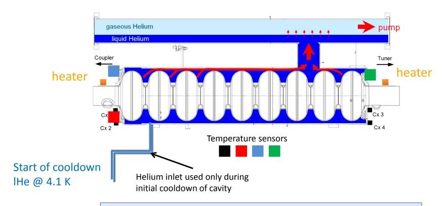
Dynamics of Helium filling leads to large temperature gradients
