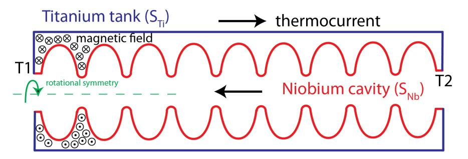
$$U_{\text{thermo}} = (S_{\text{Niobium}} - S_{\text{Titanium}}) \cdot \Delta T$$
