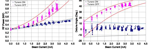
Measured and predicted RF drive amplitude and phase due to CW beam loading in an ERL where the effective current is approximately 7% of the single pass beam at 75°.
