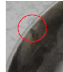
IHEP-02 quench defect (detected by second sound and thermometry). The quench location has sharp and deep grain boundary step made during half cell pressing.
