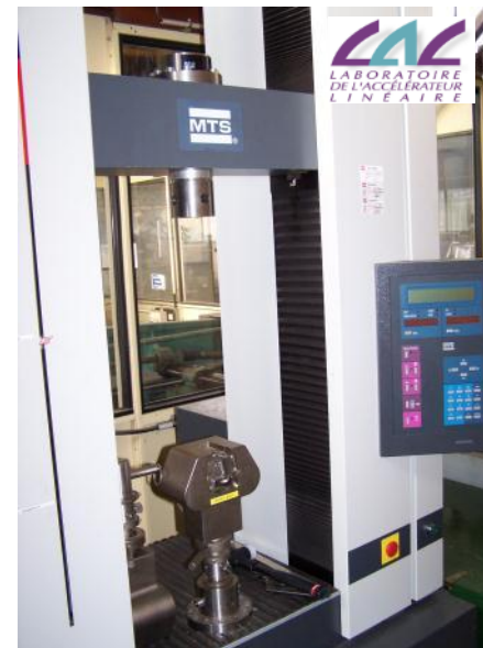
Machine de traction (force maxi 150 KN, course maxi 700 mm)
