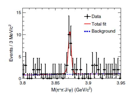
ISR  $\psi$ ' signal is used for rate, mass, and mass resolution calibration.
