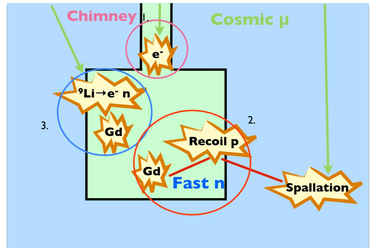
**Fast neutrons** (and possibly stopping  $\mu$ ) can be selected with the **Pulse Shape Discrimination (PSD)** using the difference in the Pulse Shape between positrons and protons (muons).
