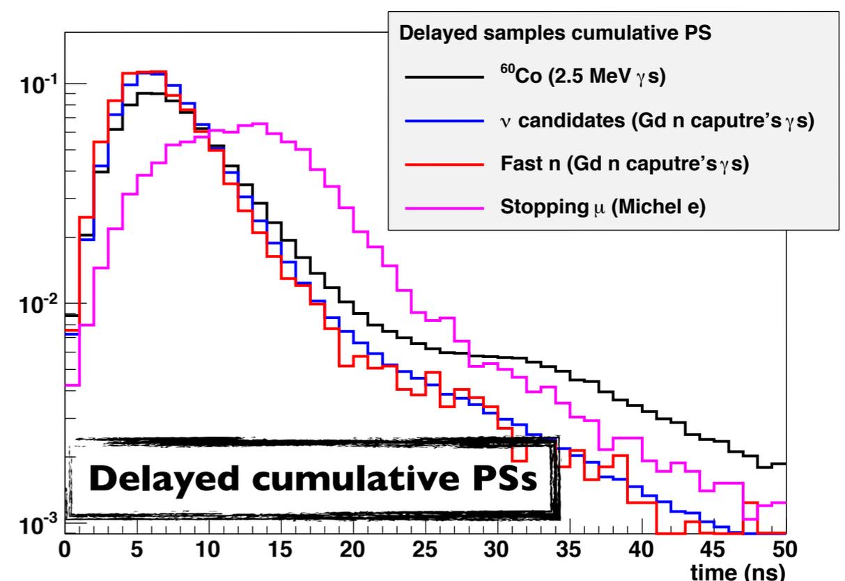
We use this differences to **discriminate Stopping Muons (Fast Neutrons) in the neutrino sample.**
