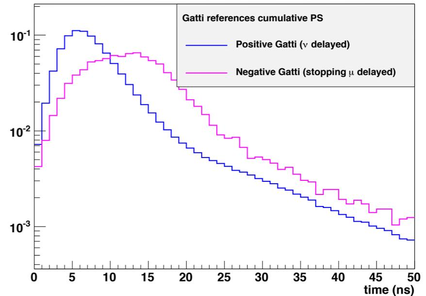
The Gatti analysis applied to “Stopping Muons” and “Fast Neutrons” separate the two populations.
