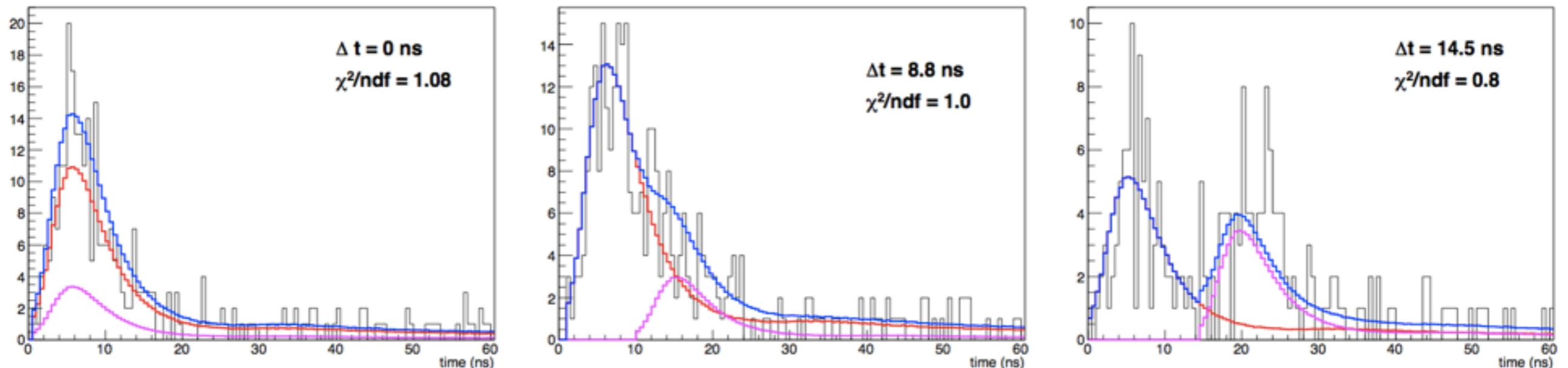
Applying the fit to all the neutrino sample we obtained a  $\Delta t$  distribution. The **formation probability and a time of life** extracted from the  $\Delta t$  distribution are **in agreement with the expected values** for the DC scintillators.
