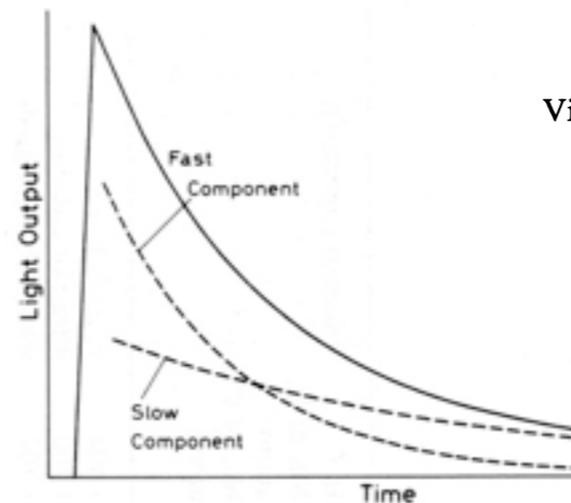
Excited state population depends on  $dE/dx$ : **higher slow component ( $\tau_3$ ) for heavy particles** (protons, alphas, ions) than for light particles (electrons, positrons, photons).
