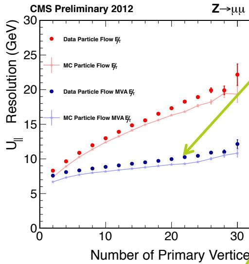
Build MVA MET to reduce degradation of resolution with pile-up
