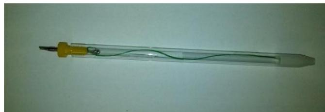
*Carbone vitreux  $\Phi = 1\text{ mm}$*
