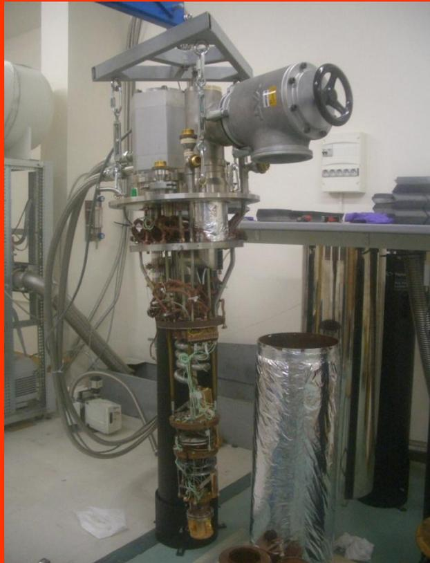
Calibration with a fixed point thermometer down to 14 mK
