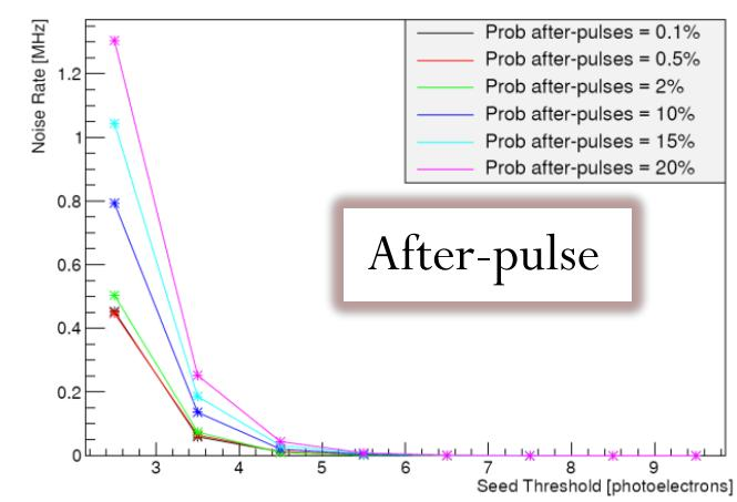
Keep after-pulse probability **below 2%** to allow for a low noise cluster rate.
