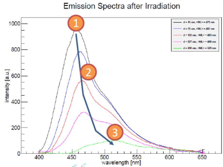
Irradiation shifts the spectrum, observed at the fibre end, towards green/red.
