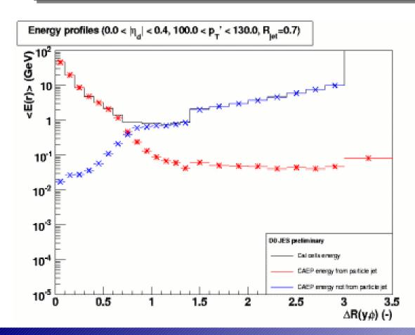
MC energy profile from particles belonging (red) or outside (blue) particle jets in y+jets events simulated at "zero" luminosity
