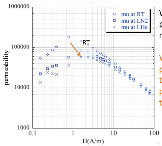
We measured the permeability of shielding material for cryogenic use.
