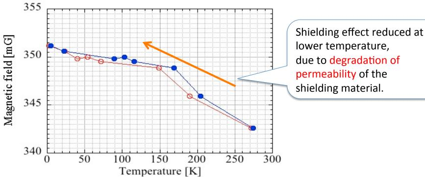
The magnetic field is plotted against both the temperature of the helium vessel (open circles) and that of the 5 K radiation shield (solid circles). A clear correlation between the shielding effect and the temperature is seen.
