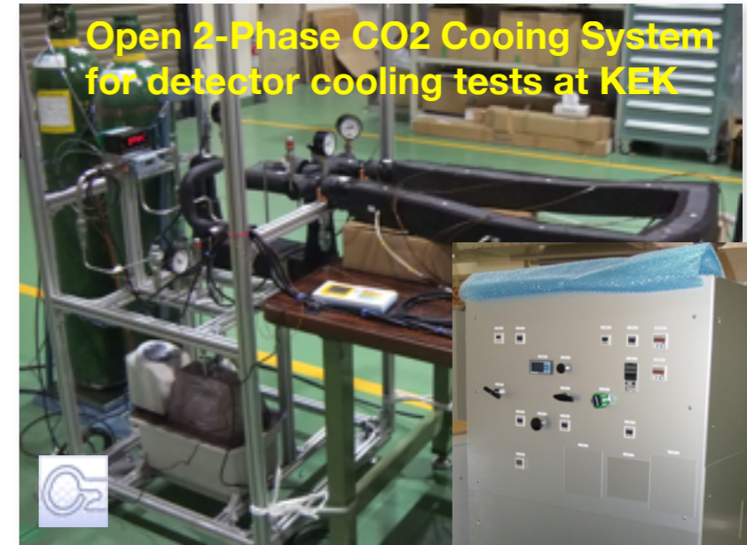
2-PCO 2 Cooling Circulation System at KEK
