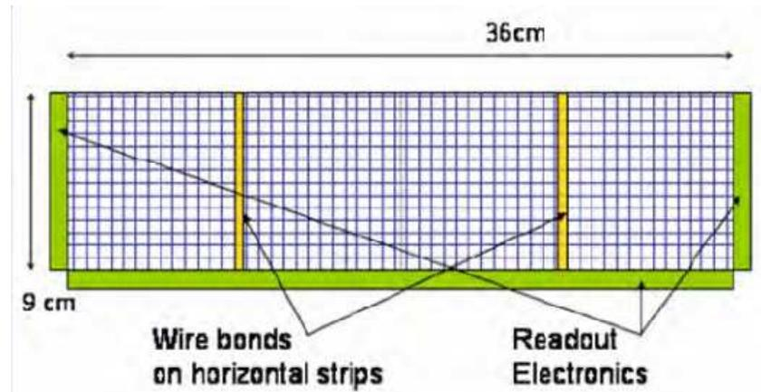
Layout of one of the four x-y tracker planes using 9 cm x 9 cm single-sided silicon detectors with one side rotated by 90 degrees.
