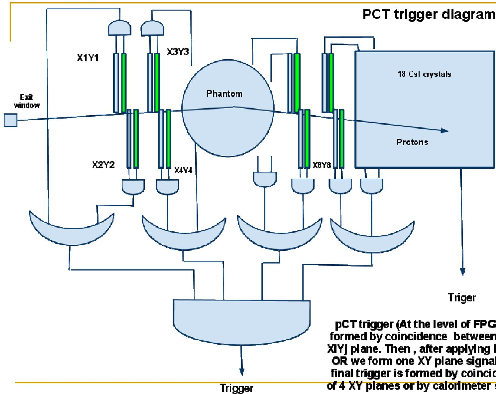
**pCT trigger (At the level of FPGA) is formed by coincidence between each  $X_iY_j$  plane. Then, after applying logical OR we form one XY plane signal. The final trigger is formed by coincidence of 4 XY planes or by calorimeter signal.**
