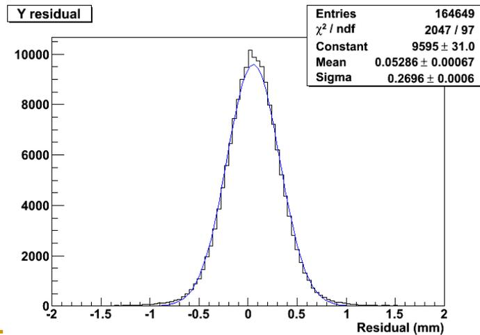
Use straight tracks from beam to calculate x and y corrections
