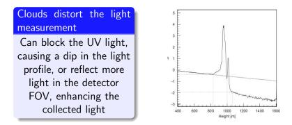
Measurements of cloud cover, altitude, and cloud optical properties can be performed with both devices. In particular, the lidar can identify multiple cloud layers. Information from vertical and inclined shots will be compared with satellite data
