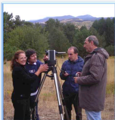
UVscope on its mount (second arm ready to support the future UV-SiPM)
