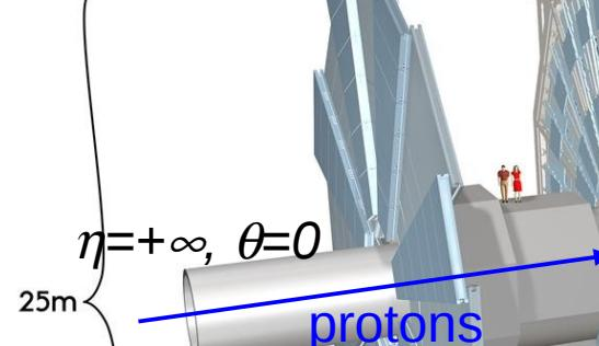
**HAD calorimeter ( $|\eta|<5$ )** : Fe/scintillator tiles (central), Cu/W LAr (fwd), Trigger, jets and  $E_T^{\text{miss}}$
