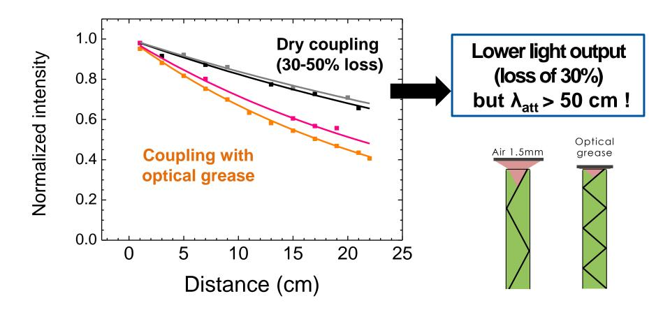
If photostatistics allow it, the selection of a narrower collection angle would improve light attenuation (within this cone).
