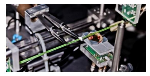
Hamamatsu 3x3mm MPPC 50x50µm
