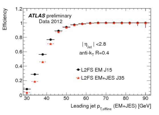
Efficiency for L2 full scan at electromagnetic (EM) and hadronic (EM+JES) calibration scale vs leading offline jet p<sub>T</sub>. Minimum jet ET thresholds are 15GeV for EM-scale trigger and 35 GeV for the EM+JES scale trigger.
