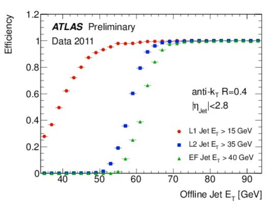
Efficiency for anti-kT jets with R=0.4 to for a jet trigger chain. Different thresholds are applied at each level of the trigger to increase rejection while keeping acceptance for events with high probability of satisfying the overall jet trigger. Results are shown with pile-up noise suppression.
