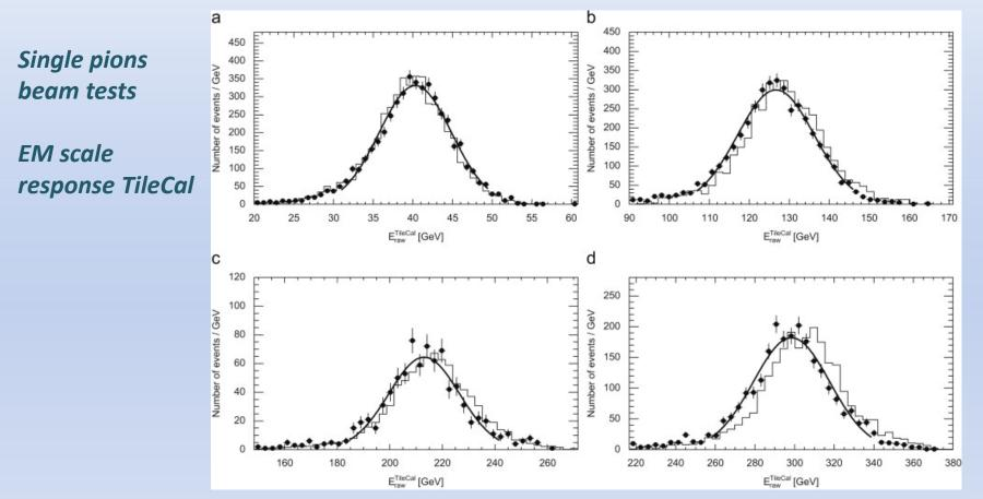
Distribution of the reconstructed energy  $E_{raw}^{TileCal}$  obtained for  $E_{nom}$  equal to (a) 50 GeV, (b) 150 GeV, (c) 250 GeV and (d) 350 GeV, and  $\eta$ =0.45. The full points represent the experimental data. The solid curves correspond to the fit of a Gauss function to the data . The histograms correspond to the prediction of the Monte Carlo simulation (model - QGSP-Bertini)
