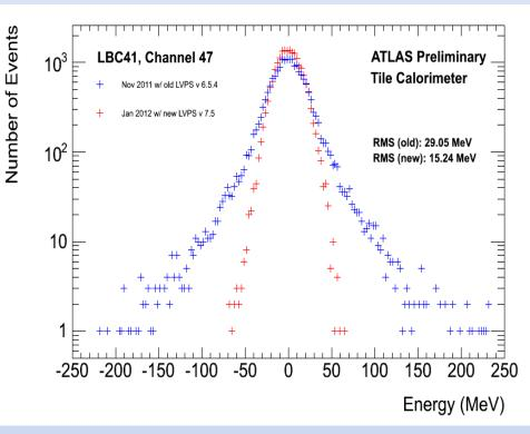
On this plot there is an example of noise for channel, which had previously high double Gaussian shape (blue). Now it is equipped with new version of LVPS (red). New LVPS also reduce correlated noise.
