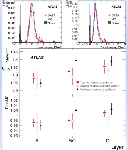
Example of the muon signal and corresponding noise for projective cosmic muons entering the barrel modules at  $0.3 < |\eta| < 0.4$ .
