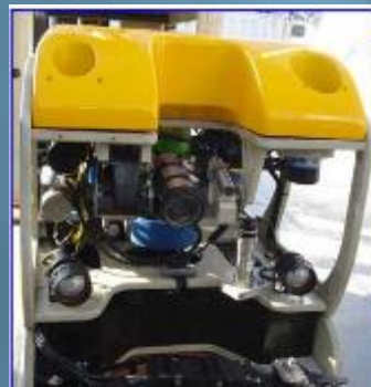
COMEX: ROV APACHE for light deep operations and connections (- 2500 m)
