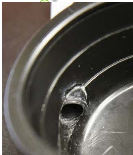
Close up of glue connection with “one second” glue.
